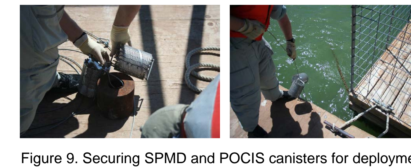
Figure 9. Securing SPMD and POCIS canisters for deployment.
