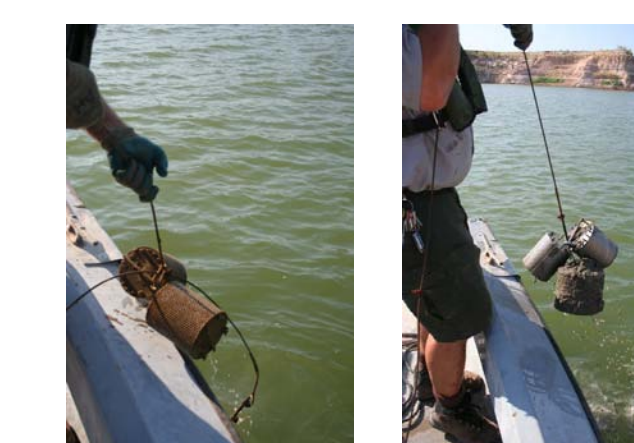
Figure 10. Retrieval of SPMD and POCIS canisters.
