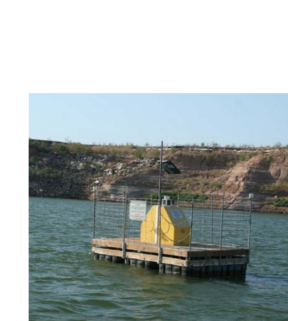
Figure 8. USGS water quality platform in Las Vegas Bay where the passive samplers were deployed.
