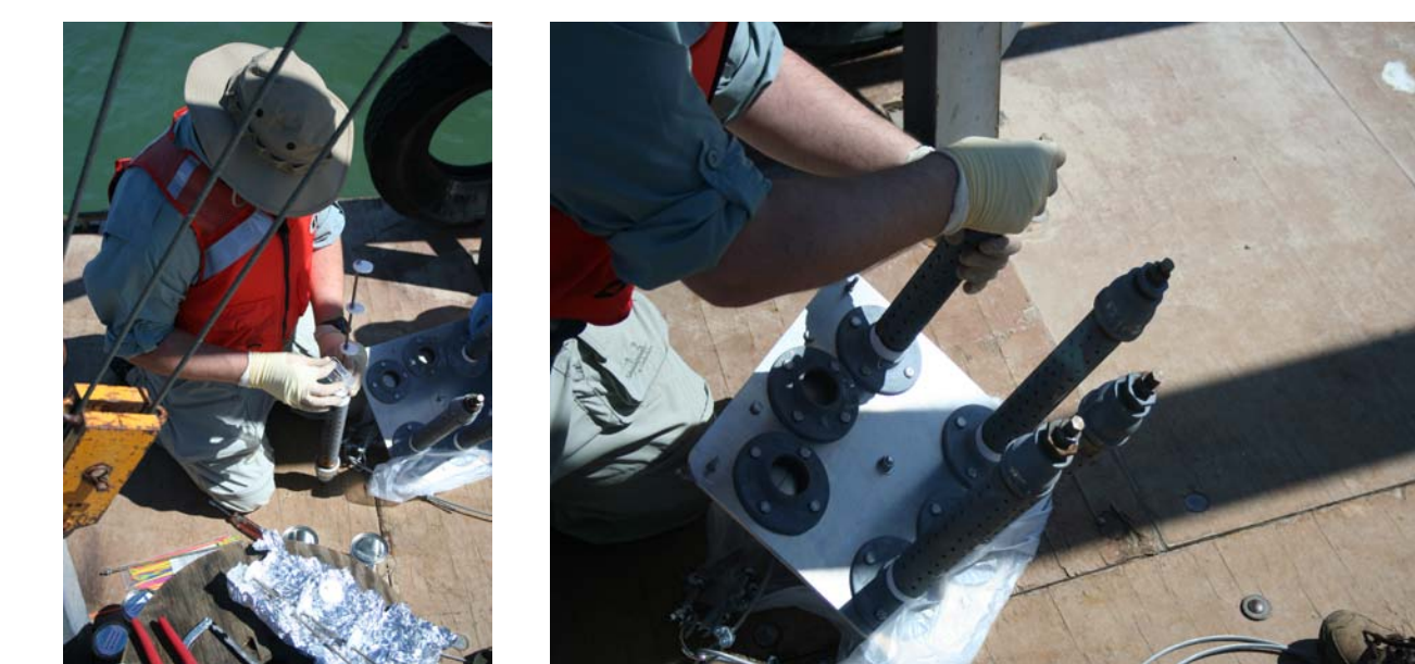
Figure 2. Assembly of the sediment probe sampling apparatus.
